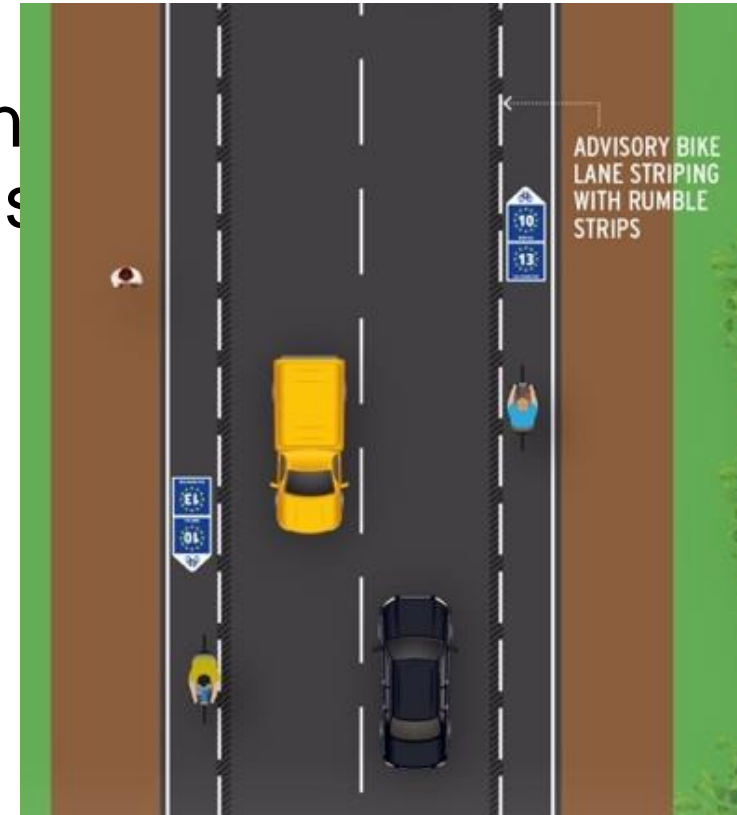
Figure 17: Cross-section with improved signing
